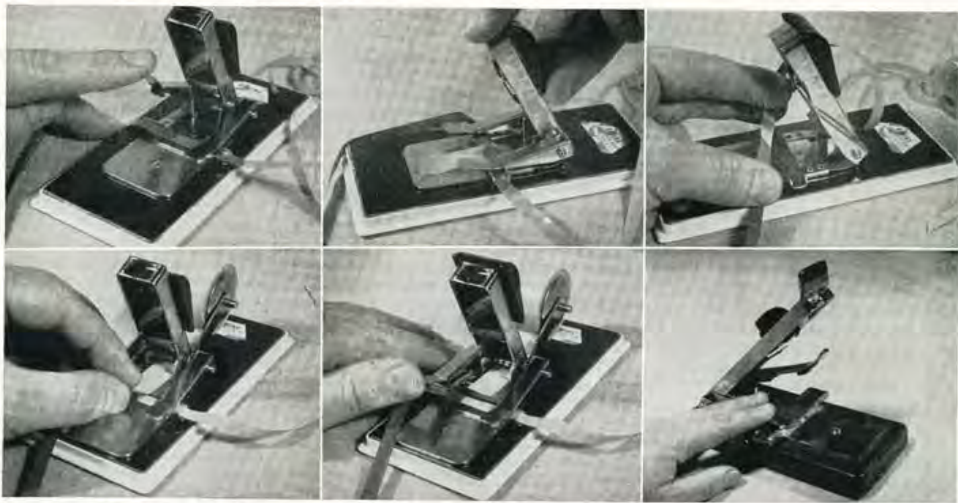
The Robins "Gibson Girl" splicer is available in several sizes and models. The tape is placed in the channels and the arms positioned to hold it. The knob is pushed back to "miter" position and pushed down. This cuts tape at 45° angle. The chip is blown away and the splicing tape applied. The knob is moved forward to trimming position and pressed down completing splice which has "Gibson Girl" shape. The unit at lower right is heavy duty model which comes in various sizes and will handle from 1/4 to 1 inch tape depending on model.
