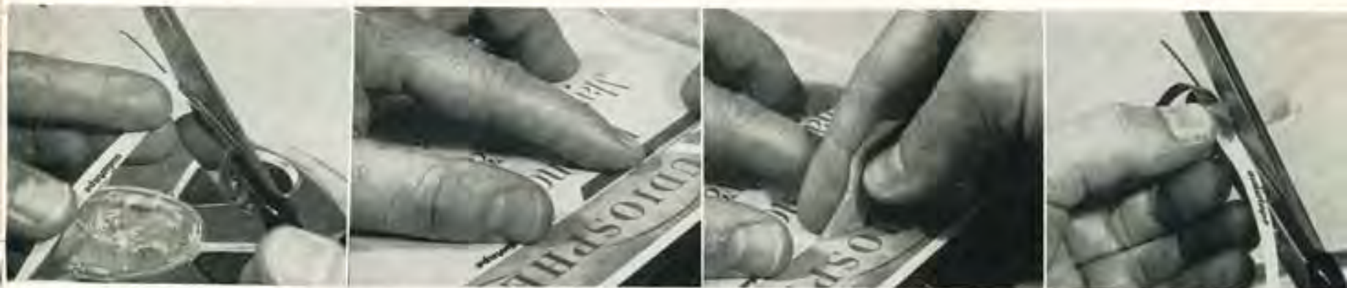
Making splices with the scissors is the most primitive method. The tape is held in alignment and a straight angled cut made through both pieces. The tape is then placed glossy side up with the cut edges butted together. Make sure tape is in line. Here printed line on box is used as guide. Apply splicing tape and press firmly. Lift splice and trim with scissors, cutting slightly into tape.
