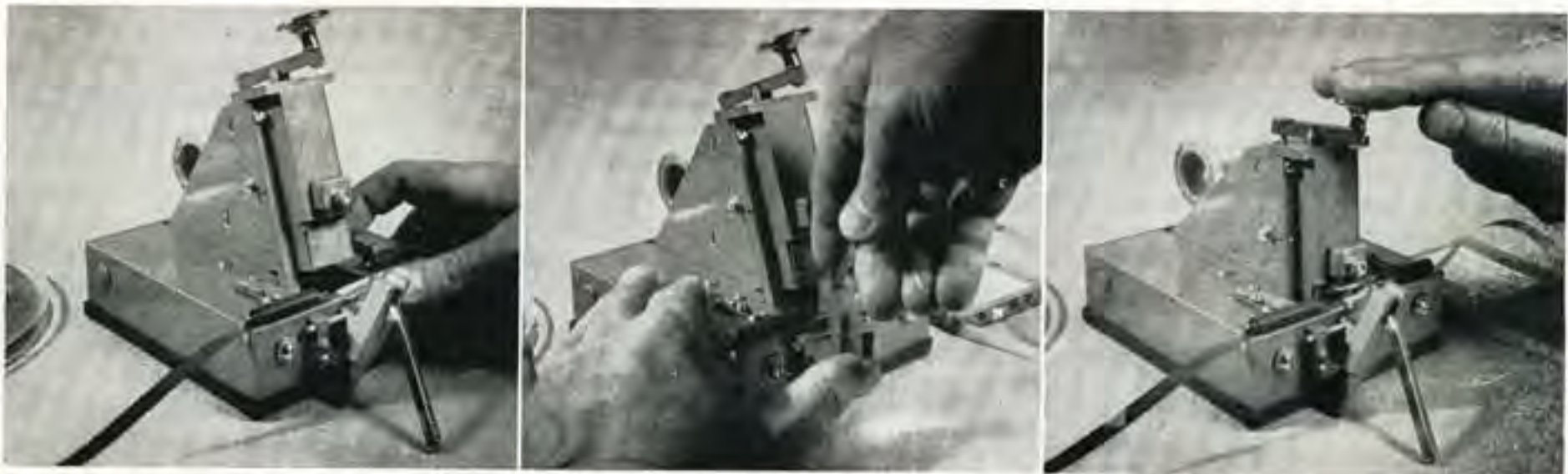
The Reiter Skila splicer automatically applies splicing tape and trims splice. The tape is positioned in the guides and rubber rollers hold it in place. The cutter bar assembly is raised and the handle pushed away or pulled toward the operator to cut tape. A carboloy wheel makes the cut. Chip is removed and the knob on top pressed. This ejects tape, applies it and trims splice all in one operation.
