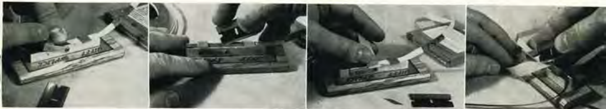
The Jiffy Splicer. The tape is placed in the grooved aluminum bar and the swinging arms are positioned to hold the tape. The razor blade is used to make the cut and the splicing tape is applied. With the tape still in the groove, the blade can be used to trim the splice before it is removed from the unit. The splicing block is mounted on wood with a felt padded base.
