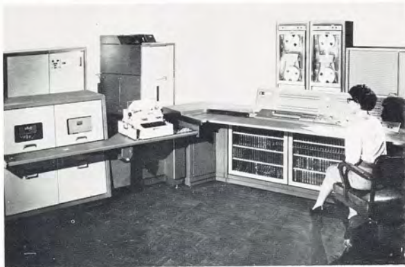
FR-300 high-speed Digital Tape Handler selected by Philco Corporation for use with new transistorized TRANSAC* S-2000 data-processing computer.
