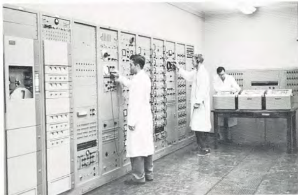
Seven-track FR-100A Recorder/Reproducer used for production-line testing of Jupiter missiles at Army Ballistic Missile Agency, Huntsville, Alabama. Photo courtesy Electrical Manufacturing Magazine
