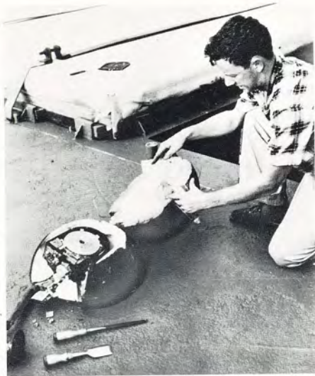
Amperex MR-100 Missile Recorders are actively contributing to this nation's missile program. Recorder shown here has been recovered from the sea after being ejected from the nose cone of a test missile.
