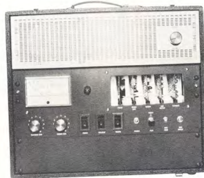
Easy front access to circuit cards, fuse and meter adjustment. Amplifier unit available without Mixer.
