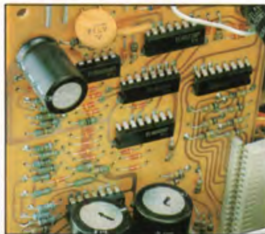
Inside the RT-909: several ICs to handle the electronic counter and the peak display.
