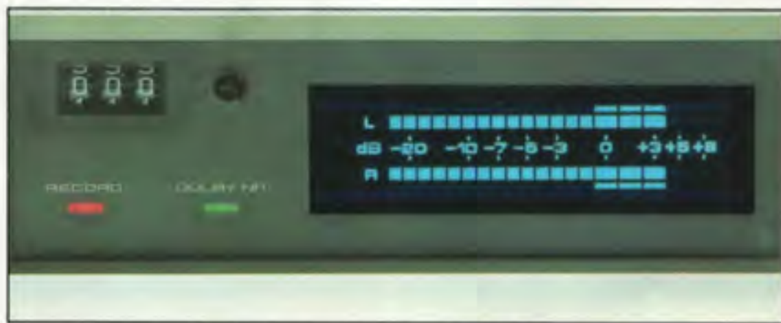
High-speed and precise fluorescent tube level meters of CT-F 600 cassette deck.
