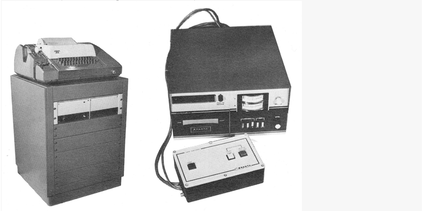
Carts were encoded for logging with the Century series record/playback machine and encoder (right). The teletype printer (left) would print out the time stamp from the digital clock, along with the five-digit code that was recorded on the cart.
