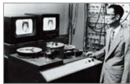
Helical scan VTR (black-and-white) developed by Dr.Sawazaki
