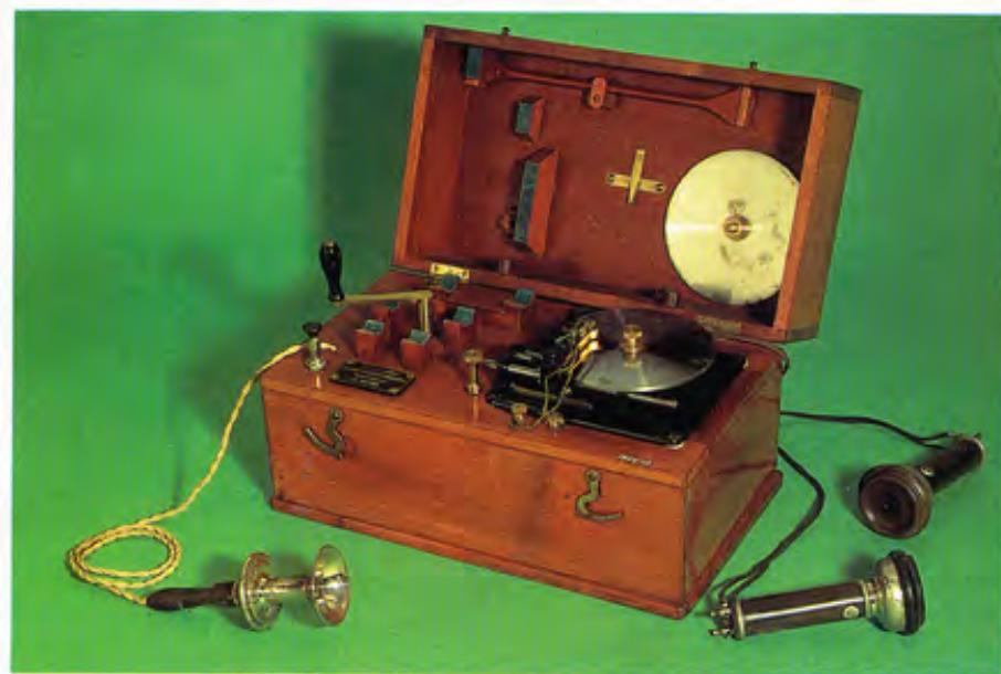
Clockwork disc-type Telegraphophone for early recording and replay —as a Dictaphone, for example
